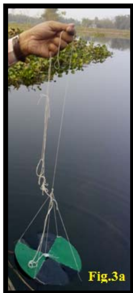
Fig.3a and 3b: Operation with Secchi Disk.
