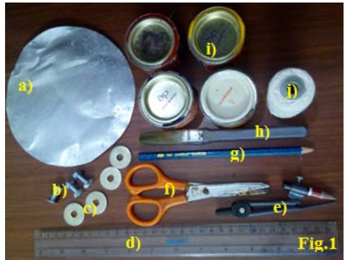
Fig.1: Materials and instruments for Secchi Disk making. a) aluminium sheet, b) nuts, c) washers, d) scale, e) compass, f) scissor, g) pencil, h) brush, i) colour paint, and j)thread.
