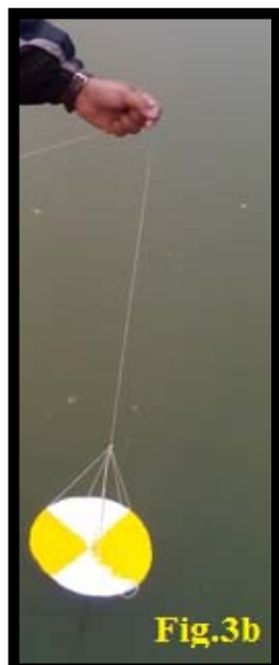
Fig.3a and 3b: Operation with Secchi Disk.
