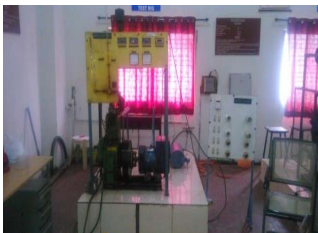
Fig 1: Kirloskar Single cylinder diesel engine
